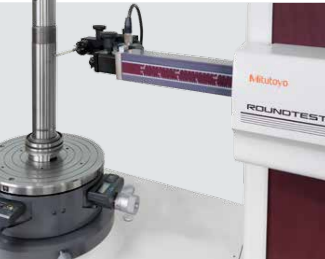
Spindle Running Test for Thermal Growth Analysis
